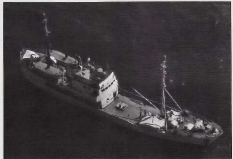
The 'Okean' class AGI Gidrofon . Most of the class have now been fitted with two positions for quadruple SA-N-5 'Grail' SAM launchers. The Barograf
